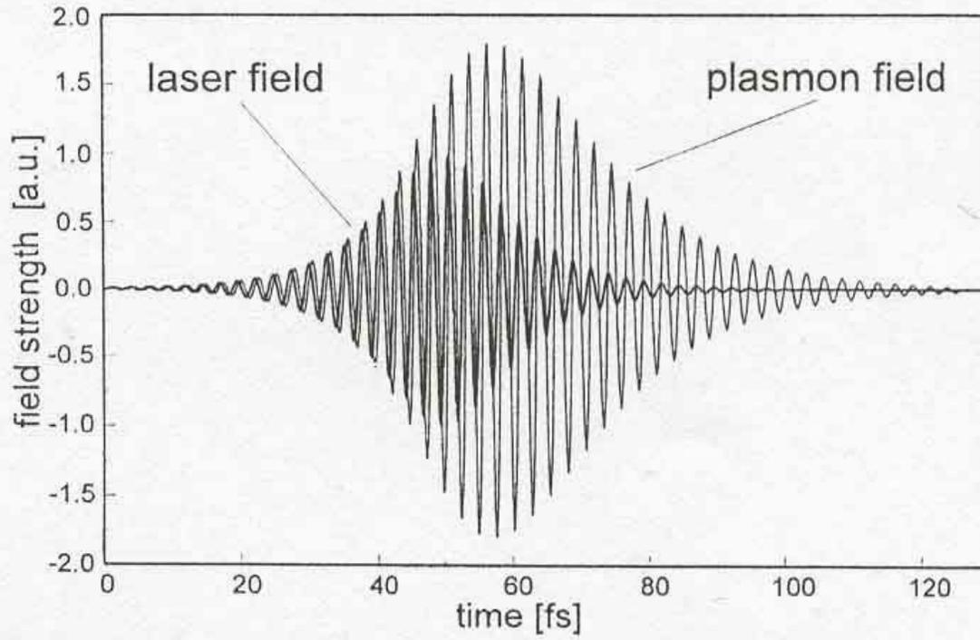
Fig. 2 Temporal behavior of the electric field  $E(t)$  (a.u.) at  $z = 0$  nm.
