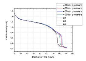
Figure 2. The voltage (V) of seven batteries versus the discharge time of each cell. Dotted/solid lines correspond to batteries discharging in air/under pressure of 400 bar respectively.
