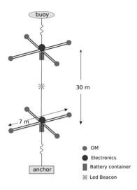
Figure 1. A schematic representation of the GRBNeT prototype detector.
