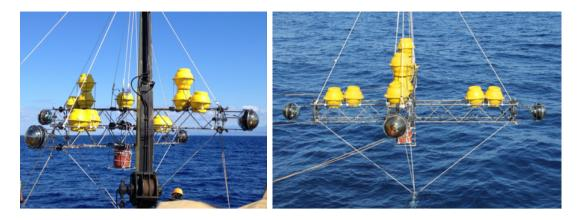
Figure 3. Left: A floor lifted from the deck of R/V AEGAEO. Right: A floor just before submersion.
