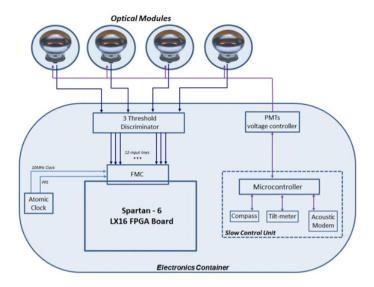
Figure 1. Block diagram of the detector unit. The prototype consists of two such units, operating independently of each other.
