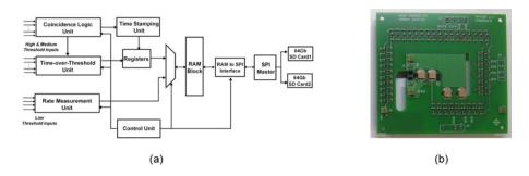
Figure 2. (a) Block diagram of the FPGA design, (b) Cockcroft-Walton board.
