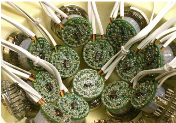
Figure 7-5: The HV supply attached to each of the photomultiplier tubes. The cables are mainly for testing purposes.
