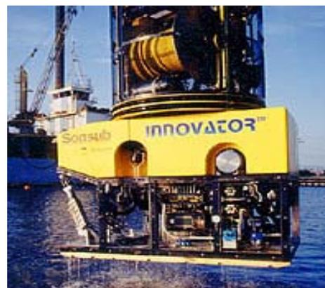
Figure 7-26: Work Class ROV.
