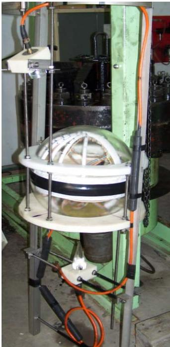
Figure 6-13: LIMS glass housing and mechanics.
