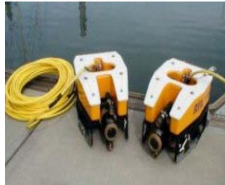
Figure 7-24: Micro Class ROV.
