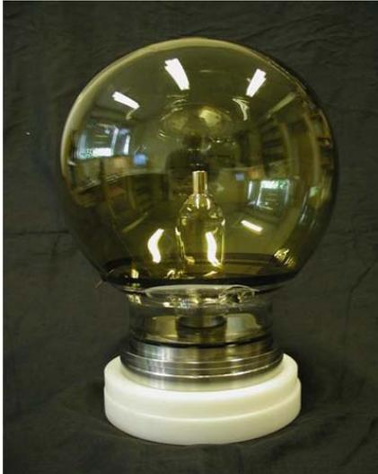
Figure 7-8: Spherical geometry X-HPD prototype, with an 8 inch diameter (CERN-Photonis collaboration).
