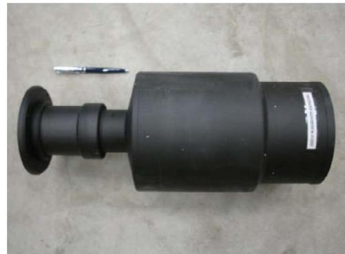
Figure 6-14: Probe for <sup>40</sup>K monitoring.
