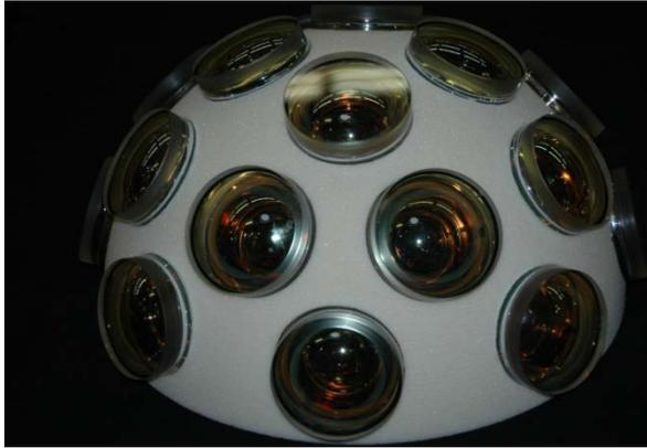
Figure 7-4: 20 3-inch photomultipliers in their Styrofoam support.
