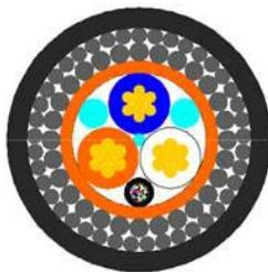
Figure 7-19: Cable option for 3-Phase AC with 3x25 mm<sup>2</sup> conductors.
