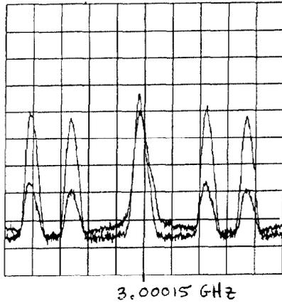
Figure 4: Horizontal Schottky sidebands in the Accumulator core betatron cooling system. Upper trace: cooling off, Lower trace: cooling on. Vertical axis 2db/div; horizontal axis span 1 MHz; the central peak is the 4471<sup>th</sup> revolution harmonic.
