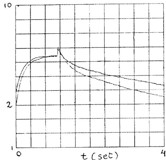
Figure 3: Horizontal emittance in the Debuncher (arbitrary units, 1 db/div) vs time. Upper trace: Notch filter off, Lower trace: Notch filter on. The sideband of the 5932'th harmonic of the revolution frequency is monitored. Beam intensity is  $6 \times 10^7\bar{p}$ .
