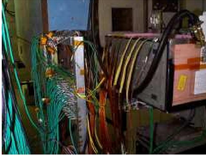
Figure 2: The moving box used to move the detectors through the beam.
