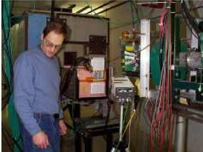
Figure 1: The booster beam area. The detectors are placed in the pink box to the right of Victor Rykalin. Above this, the beam passes through the square region and through the toroid at the right.
