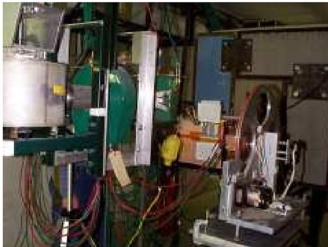
Figure 4: The Pearson 3100 Toroid which was used to monitor the particle fluence.
