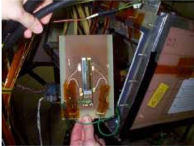
Figure 5: One of the irradiated silicon detectors showing visually that full coverage by the beam across the sensor was achieved.
