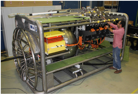
Figure 6: Photograph of a KM3NeT-France junction box (left). Schematic of the connections to the junction box (right).
