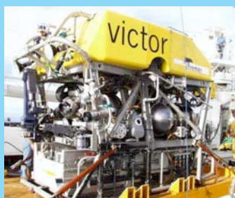
Figure 3-49: The Ifremer VICTOR ROV and a light class Seaeye Cougar-XT ROV shown at the right in its subsea “garage”.
