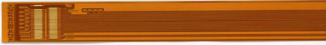
Figure 122. Digital jumper prototype cable : connector side
