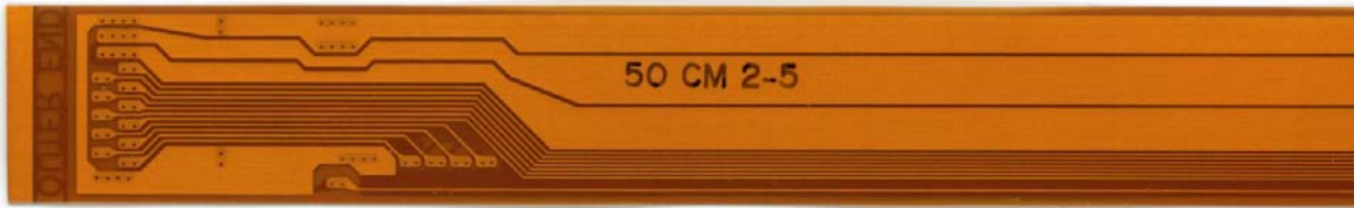
Figure 121. Digital jumper prototype cable: side opposite the connector
