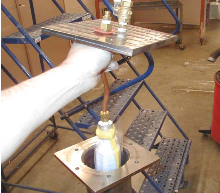
Figure 73. Loading the autoclave
