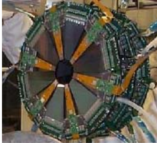
Figure 145-Mounting of radiation monitor fingers on F-disks
