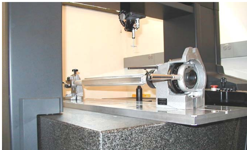
Figure 85. Index fixture with prototype mandrel
