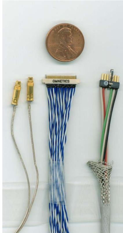
Figure 125. Prototype cables for the twisted pair assembly; from left to right : two connectors for micro-coax cables, 44-pin Omnetics connector for signal pairs, 6-pin Omnetics connector for HV and power lines.
