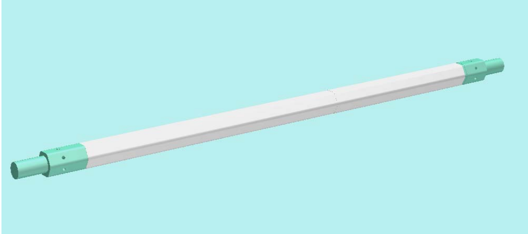
Figure 80. L0 precision mandrel with inner shell
