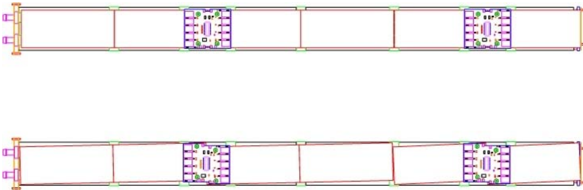
Figure 4 - Readout configuration for outer layer staves. The upper configuration is for the axial side of the stave, the lower shows the stereo side of the stave. The interaction point ( z=0 ) is at the far right-hand side of the drawing
