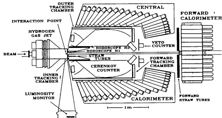
Figure 1: The E760 detector.
