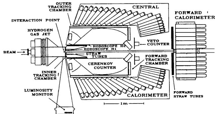
Figure 1: The E760 detector.
