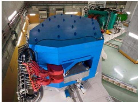
Fig. 1: The high resolution magnetic spectrometer as of spring 2008.
