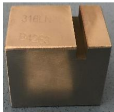
Austenitic steel for blankets
