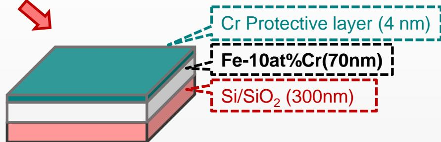
3) Verification of Cr content: X-Ray Fluorescence (XRF) and Rutherford Backscattering Spectrometry (RBS)-NCSRD
