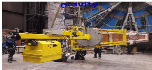
Set orientation to 22.5 deg Installation Fixation on NSW A
