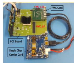
INPP DIL setup with SCC and RD53A on electrical link (Desktop-mode)
