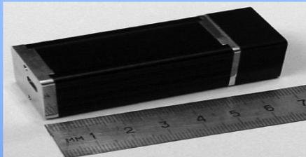
Figure 1: Solid state spectroscopic CZT detectors.
