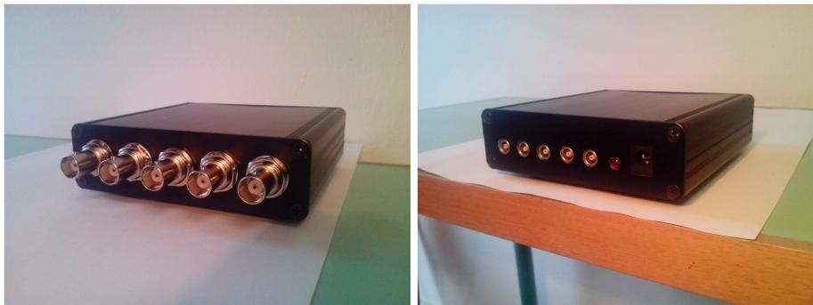
Figure 3.26: The preamplifier module: (Left) BNC Inputs, (Right) Lemo outputs
