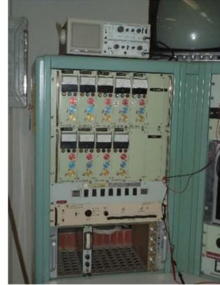
Figure C.5: (Left) Photo of the inside of the Beam Profile Monitor (BPM) depicting motor and shaft of the rotating wire. The metal shield lining the inside of the beam-line is connected to the BPM signal collector. (Right) Photo of BPM controller box (down just above Nuclear Instrumentation Module (NIM) crate) and on top the oscilloscope viewer at the Tandem control console.
