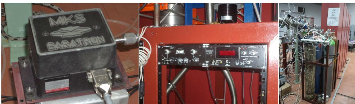
Figure 3.9: Gas delivery system. From left to right: MKS 390H pressure transducer, MKS 250E pressure controller and MKS 270D signal conditioner and last, the gas manifold.
