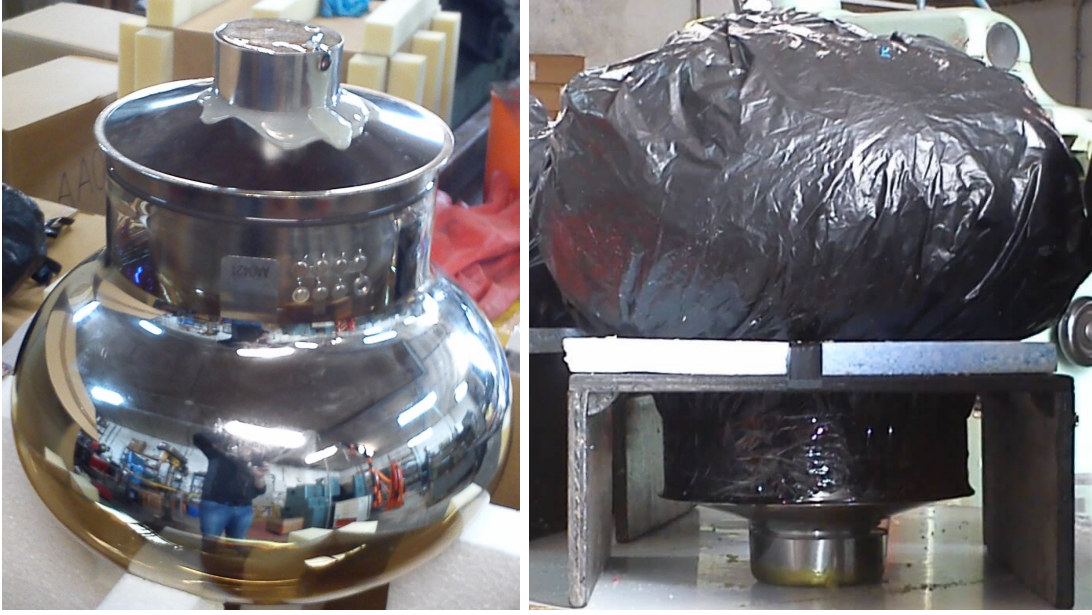
Figure 4.3: Left: A PMT with the original resistive base enclosed in the resin. Right: A PMT during the resin-removing procedure.
