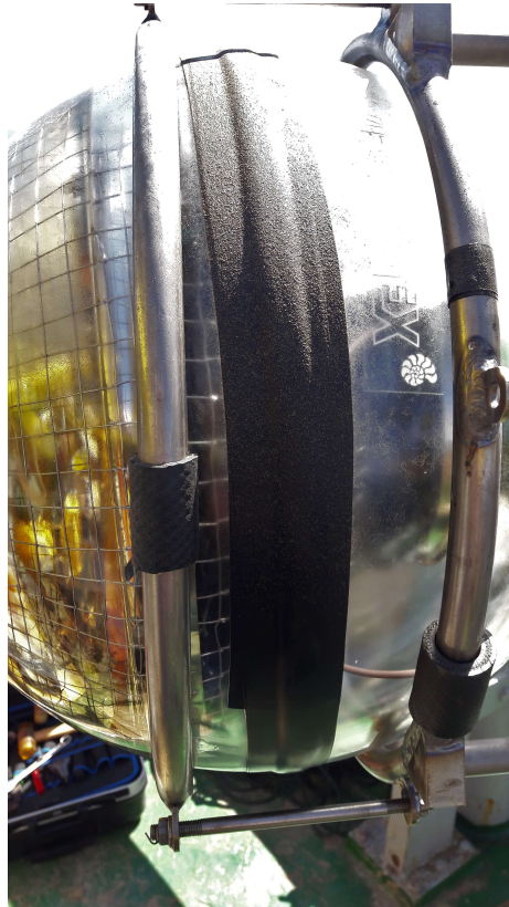
Figure 4.21: A photograph taken right after the recovery of the prototype on-board AEGAE0. The sedimentation can be observed along the scotch tape mainly on the top side of the OM, as expected.
