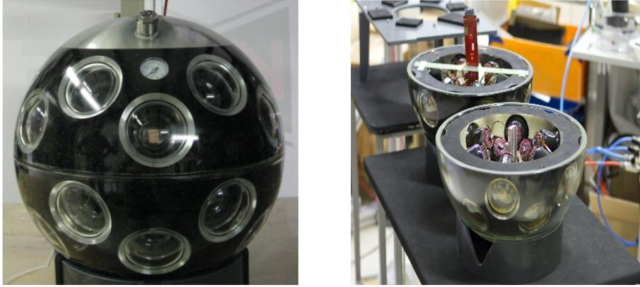
**Figure 3.8:** Left: The KM3NeT digital optical module. Right: The assembly of the prototype.
