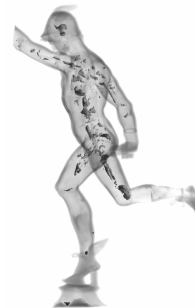
Figure 1: Example of a Mercury sculpture as reconstructed from the tomography data. It is e.g. possible to visualize and to measure the size and distribution of empty volumes with the help of specialized software tools
