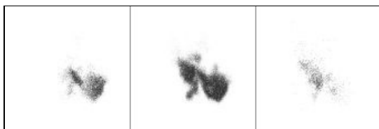
Figure 1: Fe K_{\alpha} X-ray images of an iron ore particle measured with polycapillary lens on Si(Li) spectrometer at three different distances (+50 \mu m, 0 \mu m, -50 \mu m) along the microbeam axis.
