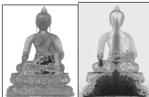
Figure 1: Comparison of the X-ray image of a Tibetan bronze Buddha sculpture (left) with the neutron transmission radiography image (right): the inner filling content becomes clearly visible because of its organic origin
