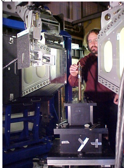
Figure 1: Sample mounting on the neutron strain scanner ENGIN-X at ISIS.
