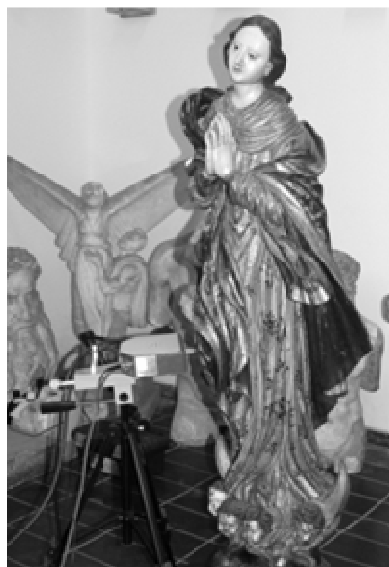
Figure 1. The analyzed sculpture and the EDXRF portable system.
